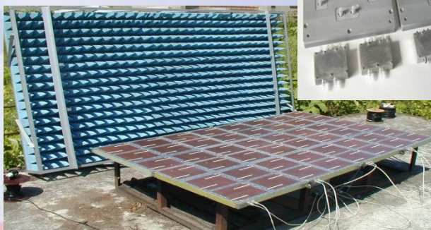
8 – channel microwave radiometer ( \lambda = 21 \text{ cm} )
