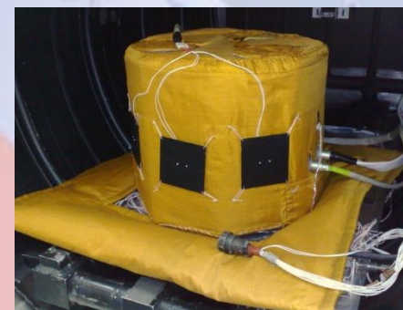
Outer detectors of Photon-Gamma apparatus in the thermo vacuum test chamber
