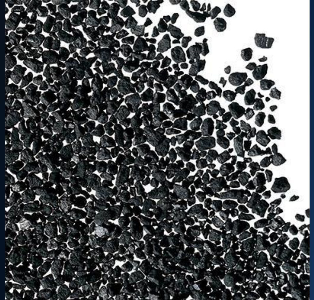
Carbon impregnated with silver ions forms the filter bed for most of Puronics' product lines. Credit: Puronics Water System Inc.
